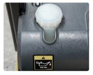
Brake Fluid Reservoir With Level Switch
