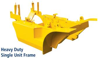
Heavy duty single unit type frame, designed on the basis of accurate structural analysis, guarantees durability and safety.
