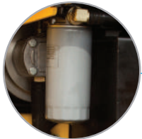
Hydraulic Return Oil Filter is Easily Accessible
