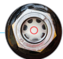
Hydraulic Oil Level Gauge
