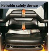
The adoption of a double safety gear minimizes the occurrence of accidents. A safety lever is to stop all functions when the operator departs from the unit; the hydraulic line is to be cut off when the key is removed.
