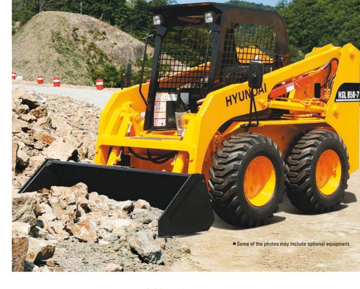
**HYUNDAI SKID STEER LOADER Applied Tier 2 Engine**
