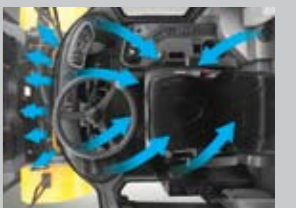
High-output air conditioner
