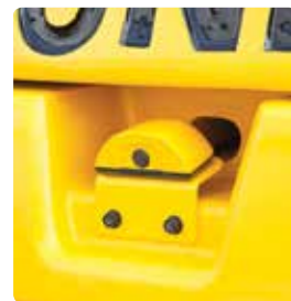
Rear View Camera (Option) The rear view camera makes the operation more easy and convenient. And it supports 4 camera channels.
