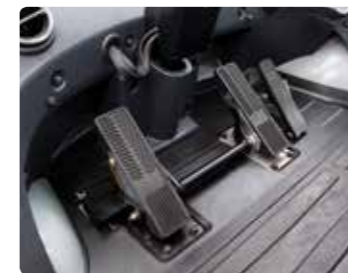
Ergonomically Positioned Pedals Based on human engineering the accelerator, brake and inching pedals are optimally positioned for the operator's convenience.
