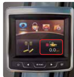
Load Indicator (Option) A load can be placed on the fork and can be accurately weighed by measuring the hydraulic pressure.
