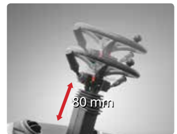
Adjustable Steering Column Steering handle is adjustable depending on the operator's body shape. Adjustability of steering column makes you more comfortable.
