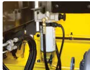
Mechanic Friendly Fuel Filter Replacement
