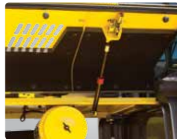
Automatic Self Locking Gas Spring
