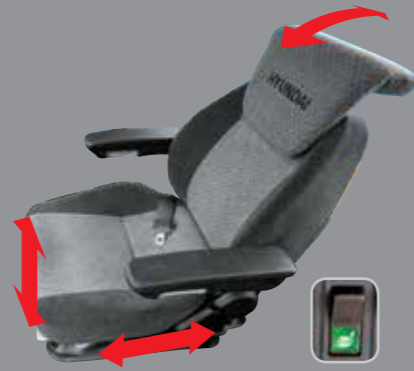
Easily Adjustable Suspension Seat
